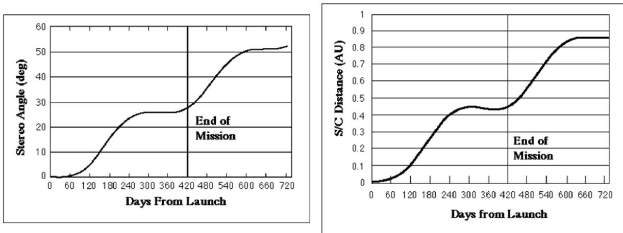
**Fig. 3: Left: Stereo (Earth-Sun-S/C) Angle vs. Flight Time** shows S/C dwells near 25° stereo angle. Right: Spacecraft distance from Earth vs. flight time.
