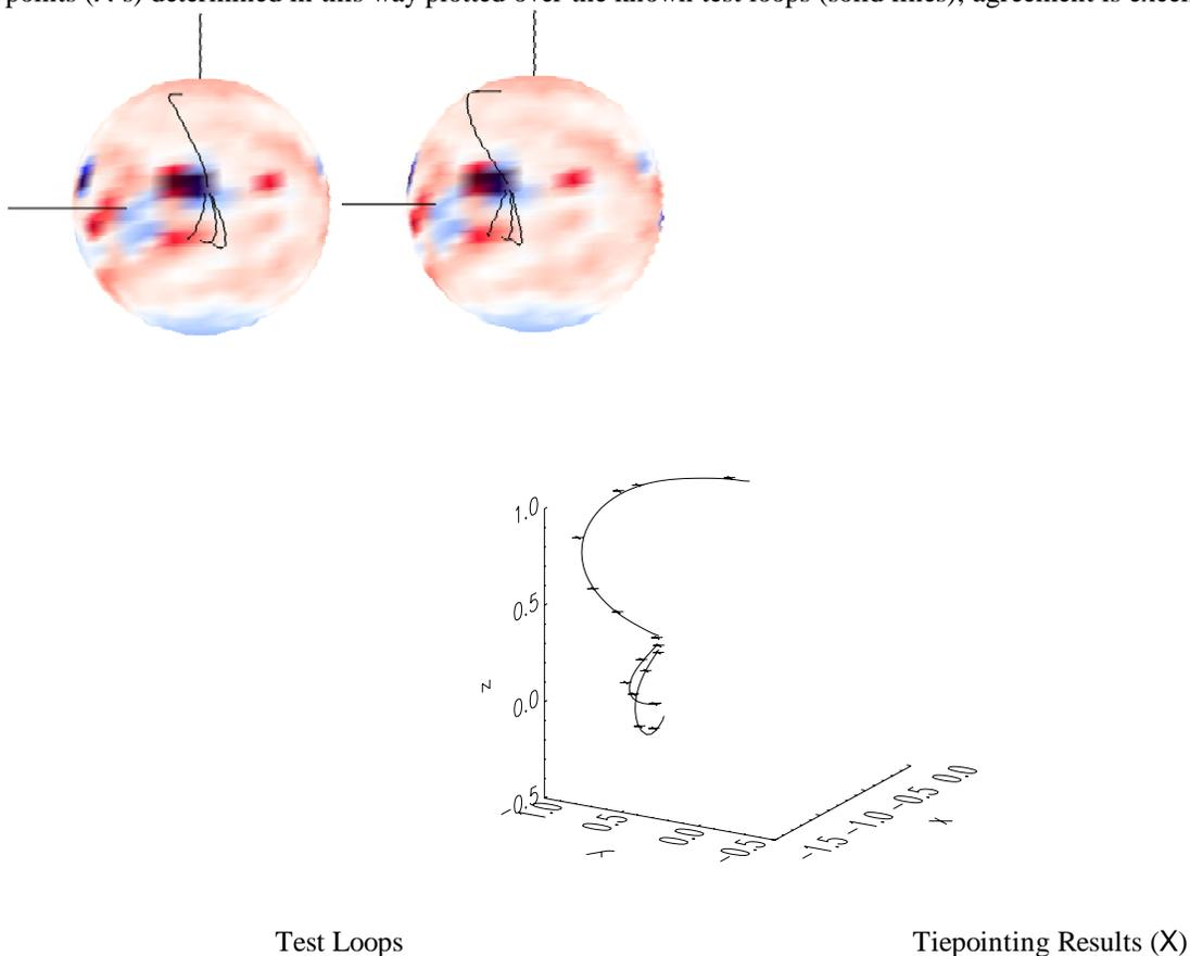
**Fig. 2. Test of determination of 3D loop geometry on known loops.** The test stereo image pair (top) was created by viewing the known loops from two angles separated by 15° (This pair may be viewed in stereo by relaxing your eye focus). The (x,y,z) location of points (X’s) determined by triangulation from the stereo pair are plotted over the known test loops (solid curves). Agreement is excellent.
